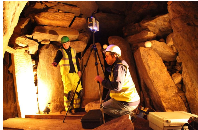
Recording the chambered tomb of Knowth using the Faro 3D terrestrial laser scanner, Discovery Programme, CC-BY-NC
